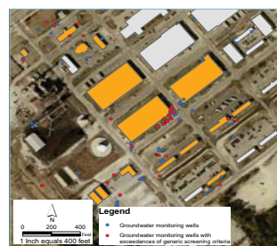
FIGURE 2 – Example Map (1 of 23 maps) Showing Buildings Located within 100 feet of Wells Exceeding Generic Screening Criteria
