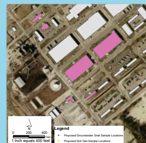
FIGURE 4 – Example Map (1 of 15 maps) Showing Phase 1 Proposed Groundwater and Soil Gas Sample Locations
