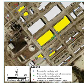
FIGURE 3 – Example Map (1 of 15 maps) Showing Buildings of Interest Located within 100 feet of Wells Exceeding Site-Specific Criteria
