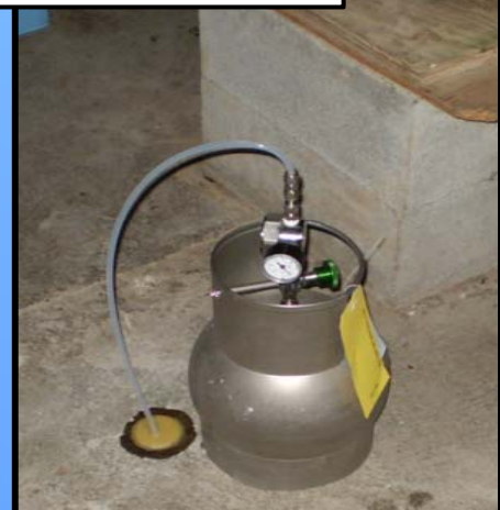
Sub-slab sample point
