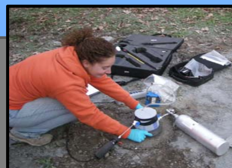
Tracer gas testing
